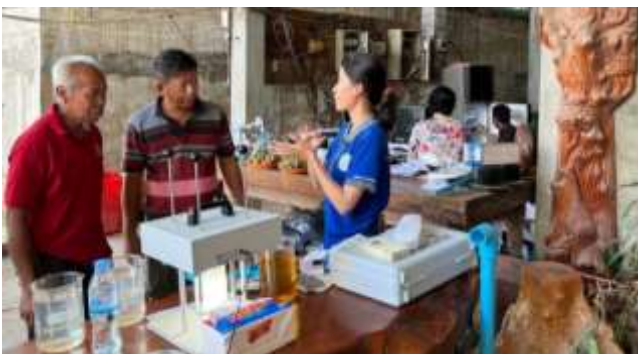
Photo 49: Raw water quality test using Jar Test at Savy Preteal Water Supply
